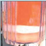
Water & bacteria in diesel oil
