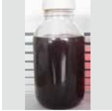
Turbine oil BEFORE filtration with the VRU
