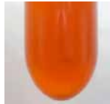
Ultra Centrifuge test, sample after a single pass through the VRU (outlet)
