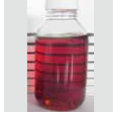
Turbine oil AFTER just a few weeks of filtration with the VRU
