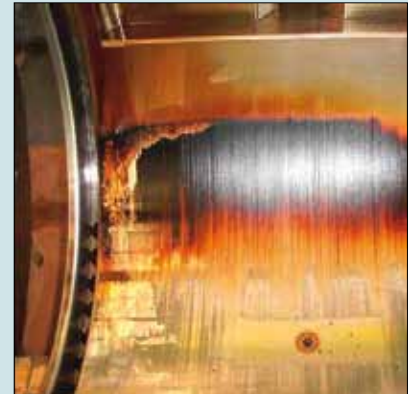
Varnish on journal bearing, gas turbine
