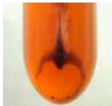
Ultra Centrifuge test, initial sample before the VRU (inlet)
