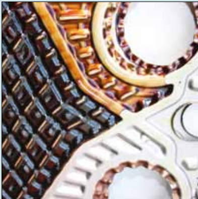
Varnish on plate heat exchanger
